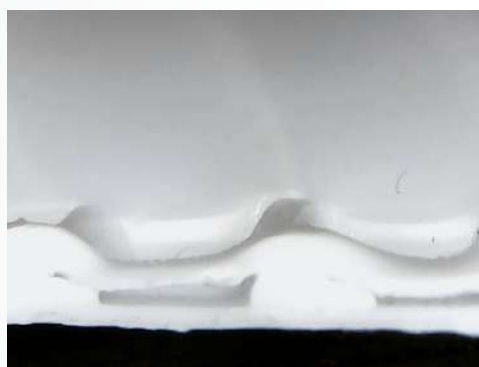
FIG.2 200X magnification of a seal performed with traditional hot-die cutting machine. Alveolar sheet in PP 3 mm thick e weight of 600 gr / m2.
